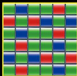
The high aperiodicity (randomness) of the arrangement of pixels in 6x6 sets reduces the occurrence of moiré. Also the presence of an R, B and B pixel in every vertical and horizontal pixel series minimizes the generation of false colors and delivers higher color reproduction fidelity.
